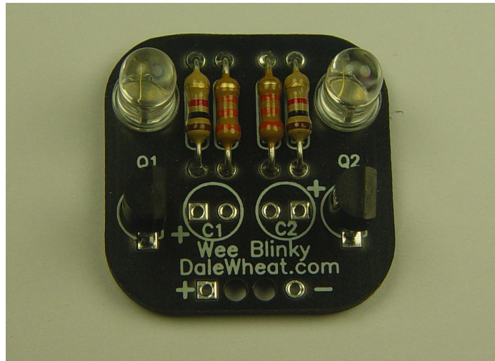
Photo 16. The LEDs are installed flush against the PCB.
