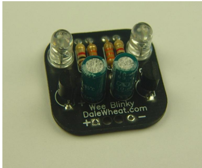
Photo 20. The right way to install the capacitors.
