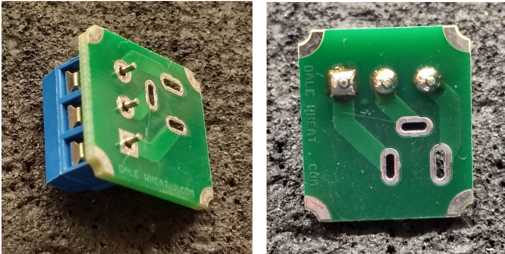
Figure 3. Install the terminal block, then solder the three pins
