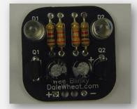
Photo 1: A properly assembled Wee Blinky
